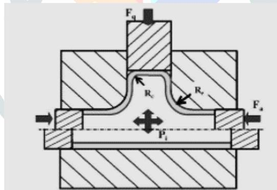
**Figure 3: Tube Hydroforming Process**
