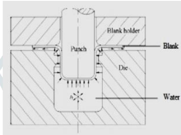
**Figure 2: Sheet Hydroforming Process**
