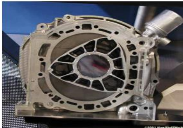
Figure1: The Rotor and Housing of a Rotary Engine from a Mazda RX-7
