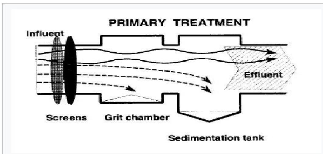
Figure 1: The basic illustration of waste water treatment through Primary treatment[7].
