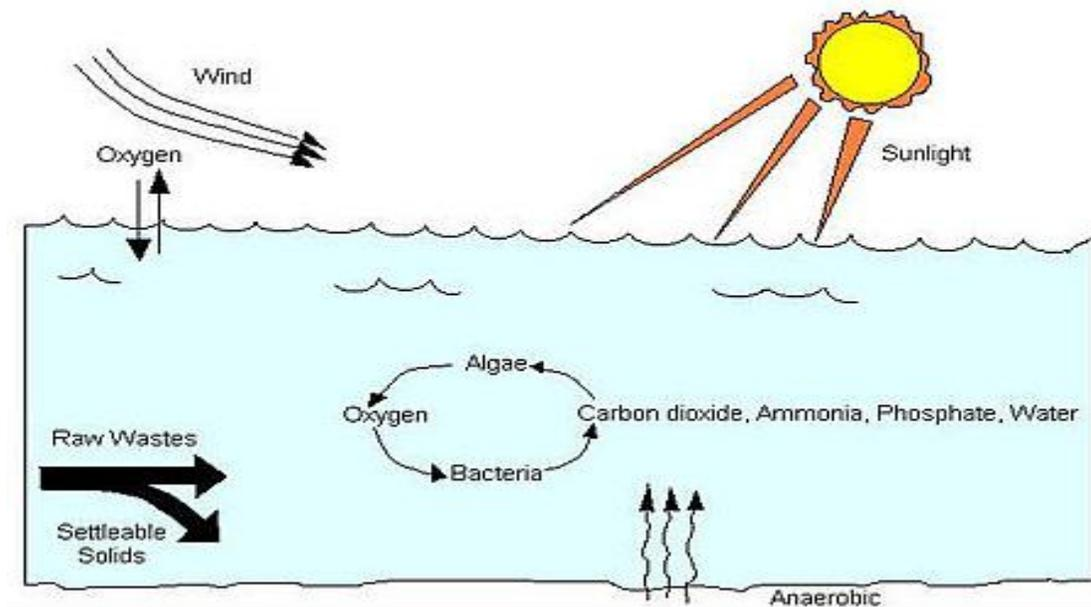
Figure 5: The basic illustration of waste water treatment through Oxidation Pond[9].
