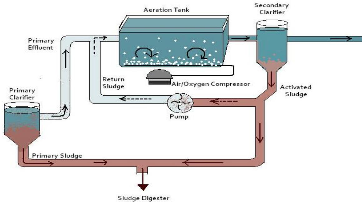
**Figure 4: The basic illustration of Activated sludge treatment of waste water[8].**
