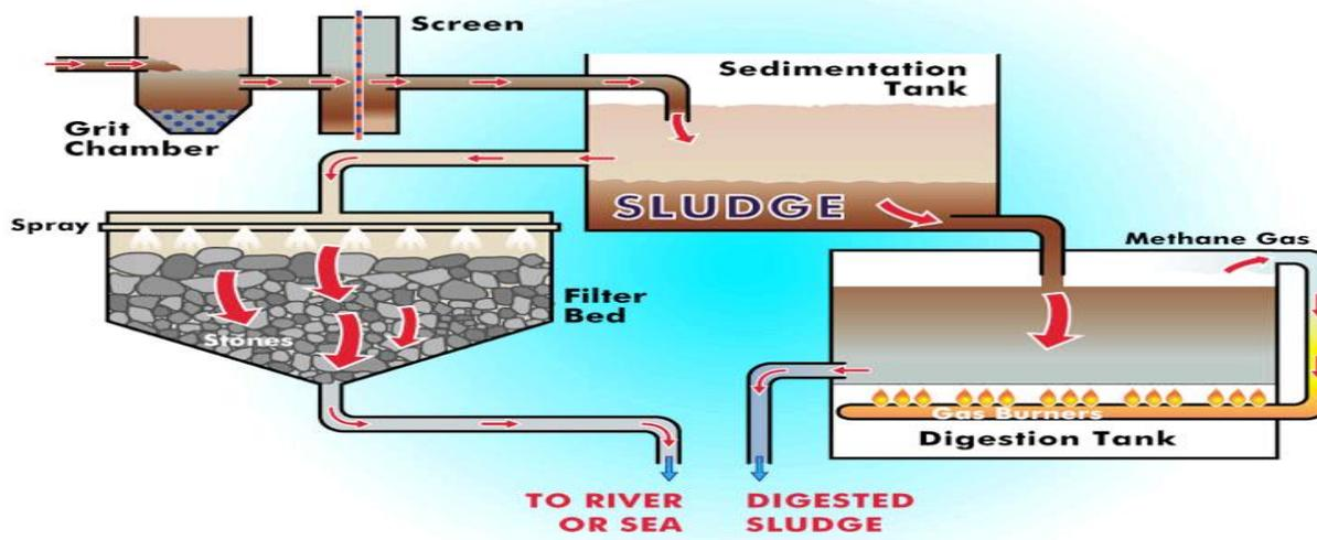
**Figure 2: The illustration of a waste water treatment through secondary treatment.**
