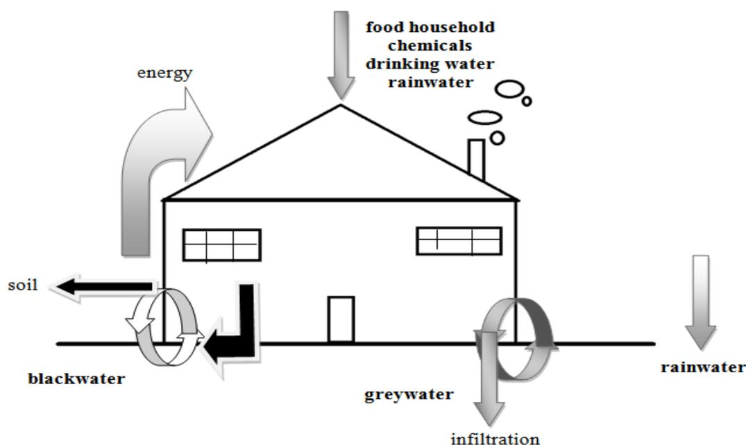
**Figure 2 : An on-site water storage facility focused on the principle of source separation, individual wastewater fraction treatment, and valuable resource recycling and reuse.**
