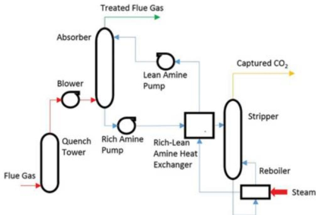
**Figure 3: Soluble amine-based absorption captures carbon dioxide from flue gas. In coal-fired advanced gasification integrated cycle power plants pre-combustion capturing could be employed [Power-Eng /Optimizing post combustion carbon capture].**
