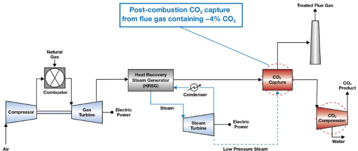
**Figure 2: Process diagram of capturing carbon. There exist three forms i.e., after combustion, pre-combustion, including oxy-fuel capture systems, which include different combustion processes [3].**
