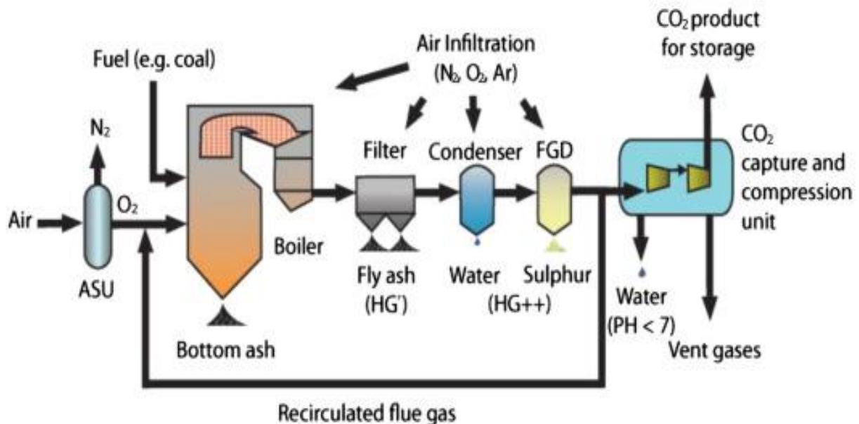
**Figure 4: Illustrates the Oxy-fuel combustion system. Oxygen is used for combustion in oxy-fuel combustion [5].**
