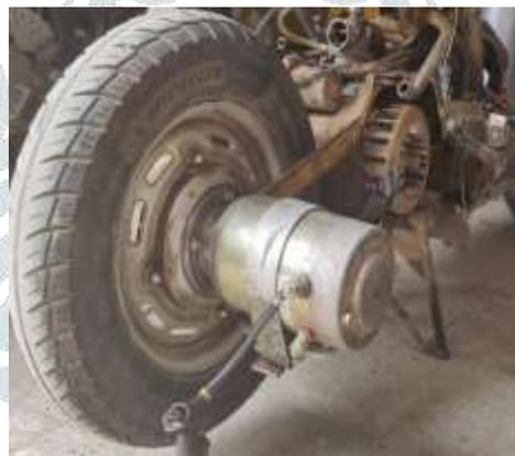
Fig.3 BLDC motor installation
