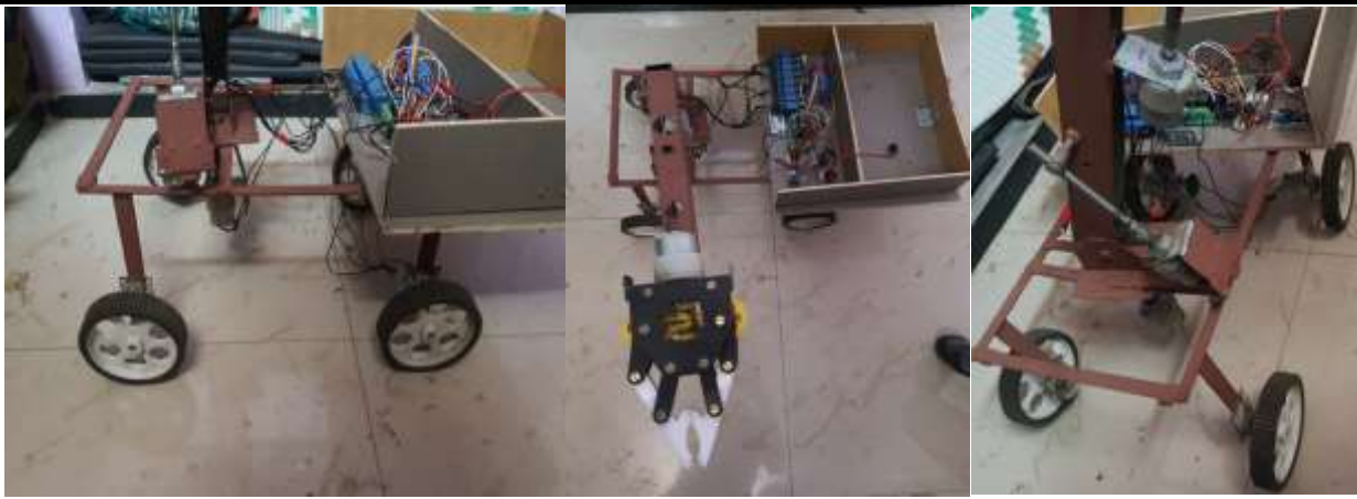
Fig.2 Wheel, Arm and gripper arrangement
