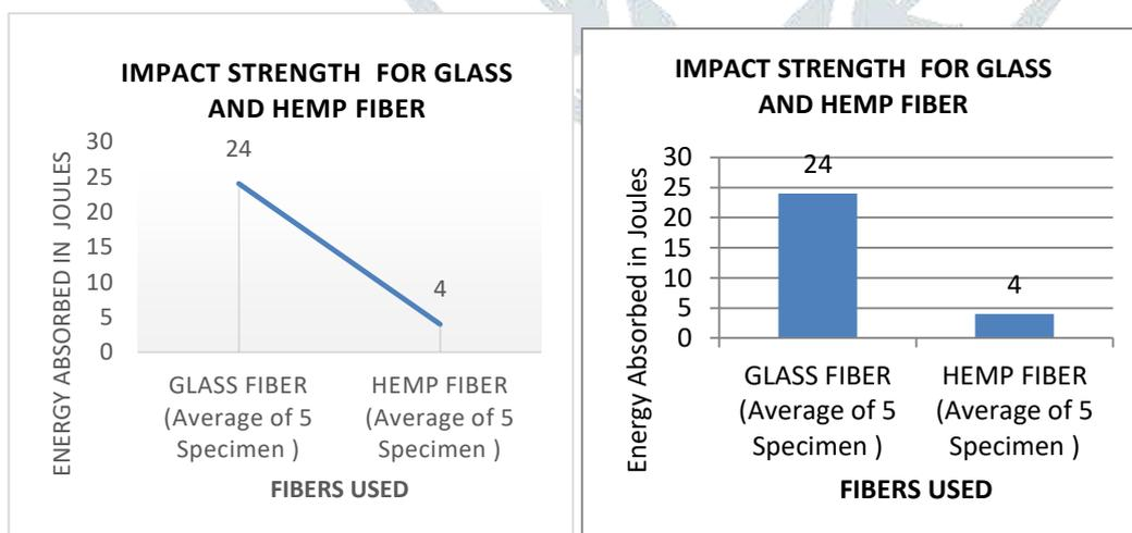
**Fig 7. Line and column graph for impact strength**
