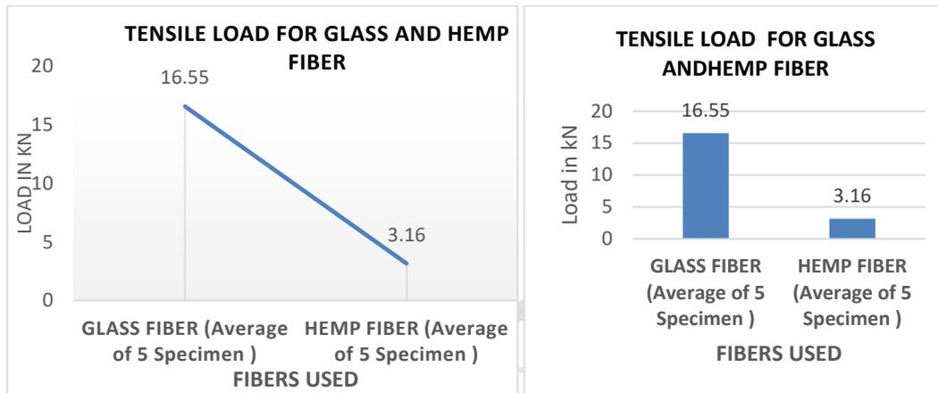
Fig 8 . Line and column graph for tensile load
