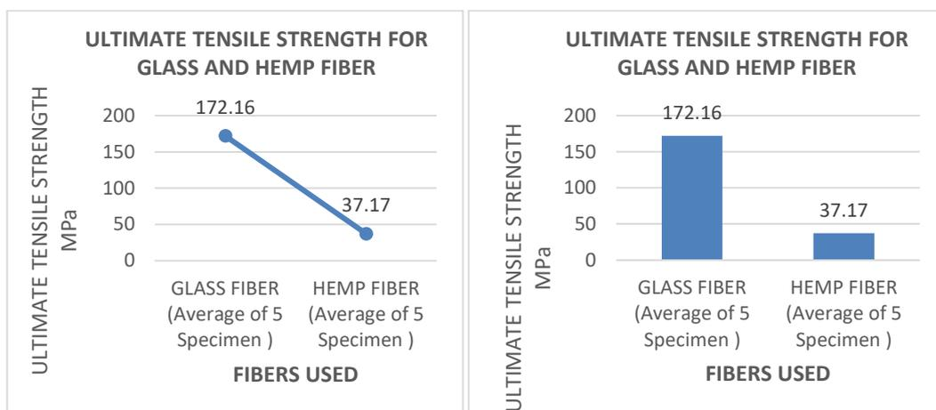
**Fig.6 . Line and column graph for tensile test**
