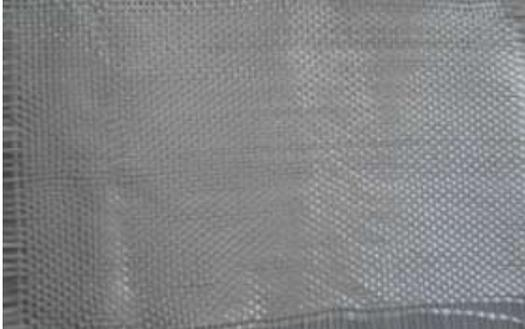
Figure 1. Raw glass fibre
