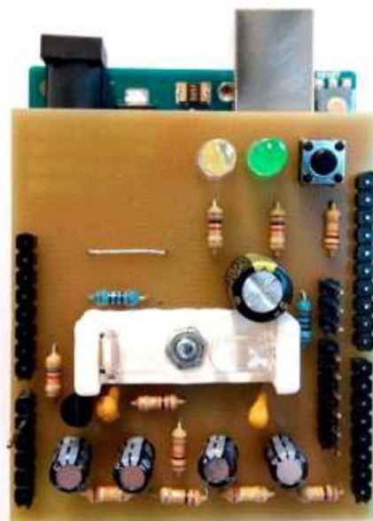
Fig. 1. Shield board for Arduino
