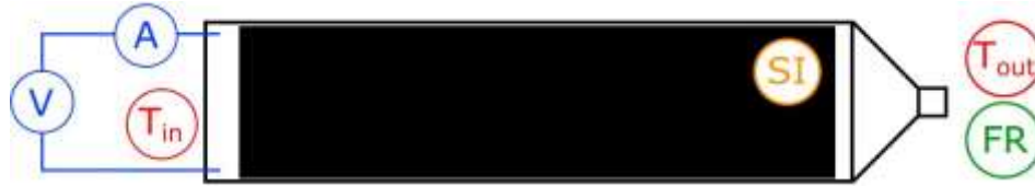
FIGURE 2: test bench schema, showing different measuring points
