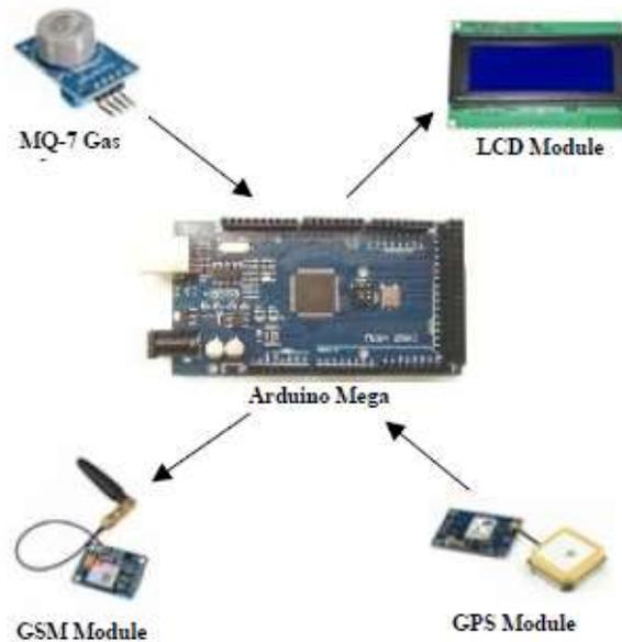
**FIGURE. 1.** Air pollution sensor diagram.
