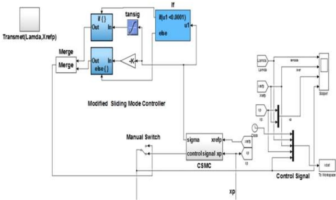
Figure 3: Block Diagram of MSMC simulation
