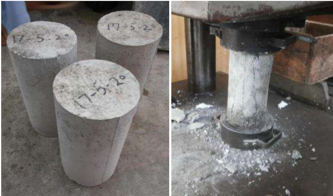
Figure 2: Concrete specimens testing in lab
