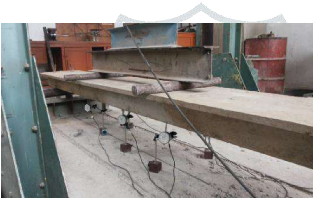
Figure 6: Loading setup for recording of deformation
