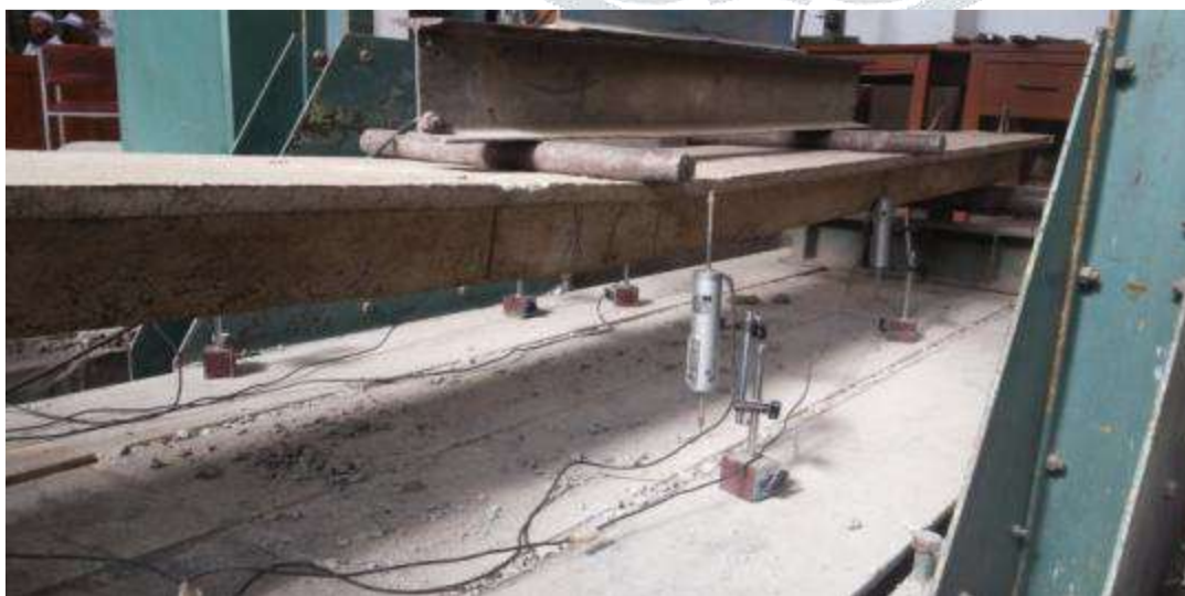
Figure 7: Ductile behaviour of panels when loaded
