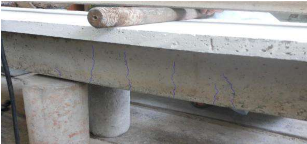
Figure 10: Cracks pattern under loading
