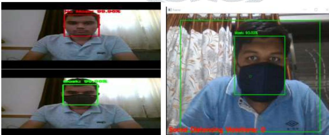
C] Model implementation :- The machine makes use of raspberry pi4 with a digital digicam to routinely monitor public areas in real-time to save you the unfold of Covid-19. The skilled version with the custom facts set is set up within the raspberry pi4, and the digital digicam is hooked up to it. The digital digicam feeds real-time motion pictures of public locations to the version within the raspberry pi4, which constantly
