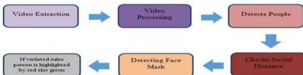
Real-time character detection is accomplished with the assist of Single Shot item Detection (SSD).A bounding field may be displayed round all and sundry detected. We after that calculate distance among all
