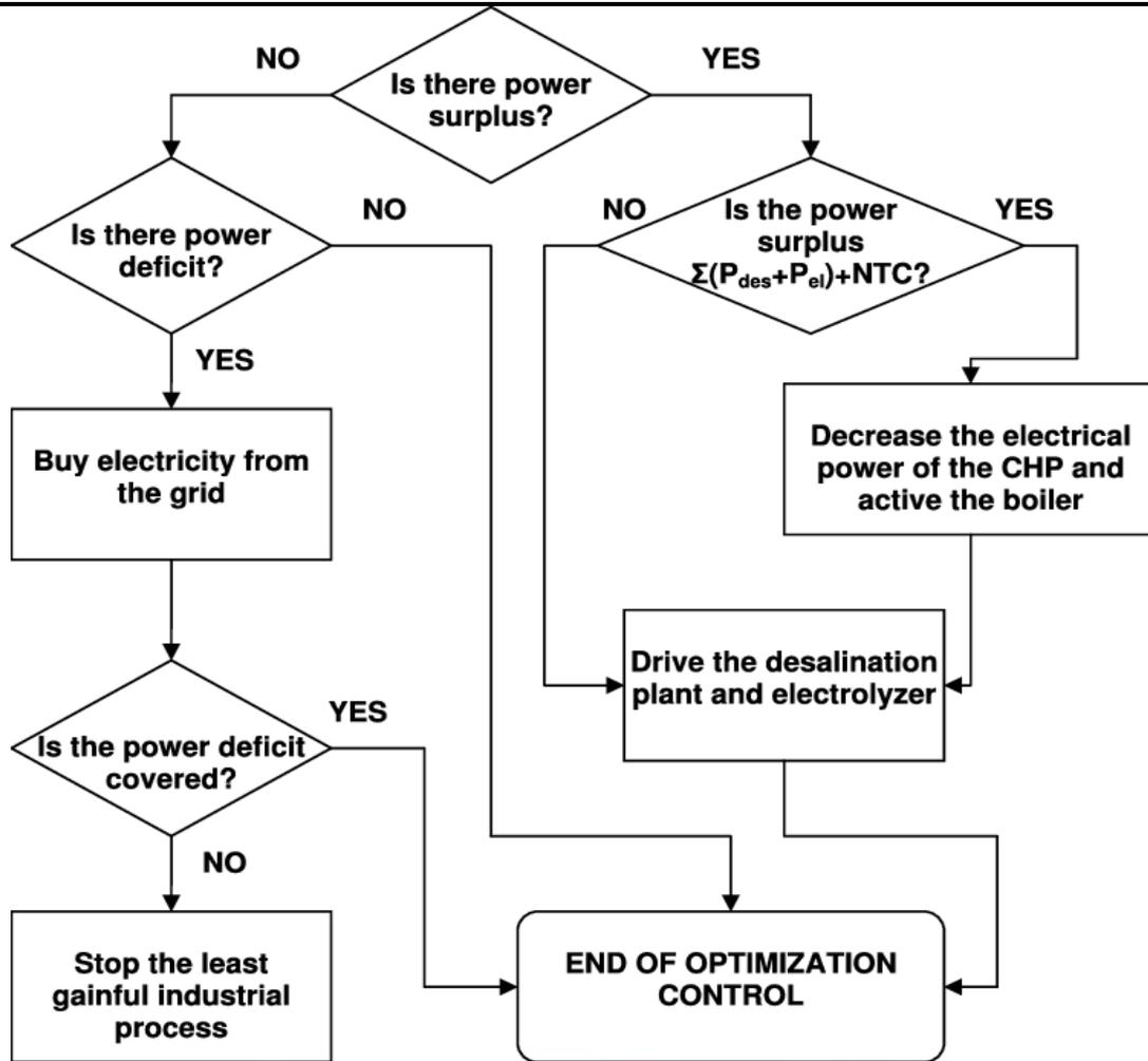
Figure 2: This diagram showing the flow chart of virtual power plant.
