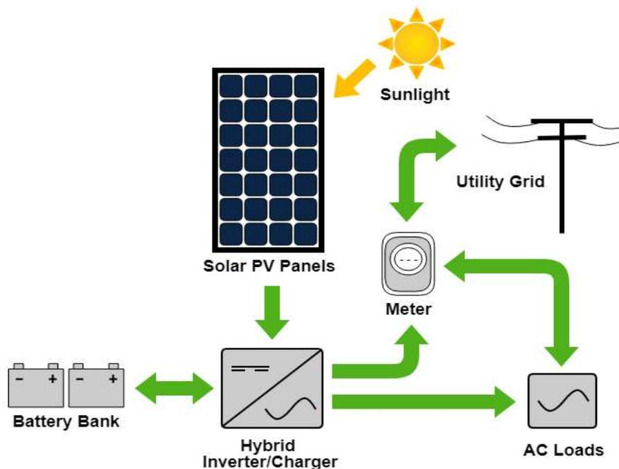
Figure 3: illustrate diagram showing photovoltaic System[9].
