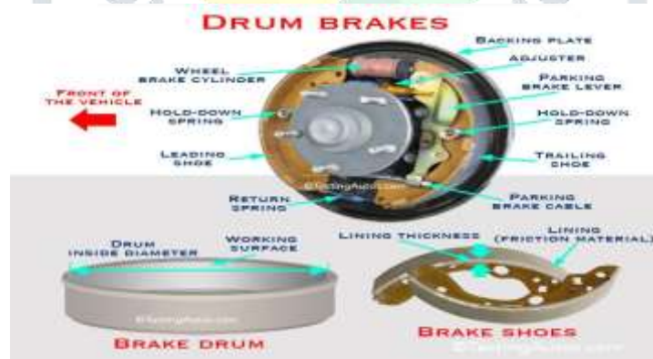
Fig. 7: Drum Brake in which Actuation Mechanism Contracts the attached Brake Shoes when the Brakes are Applied.
