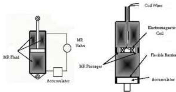
**Figure 1: Illustrates the MR fluid based Semi-Active Suspension[10]**
