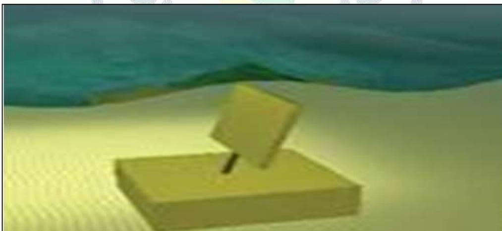
**Figure 3: Oscillating wave surge converter**
