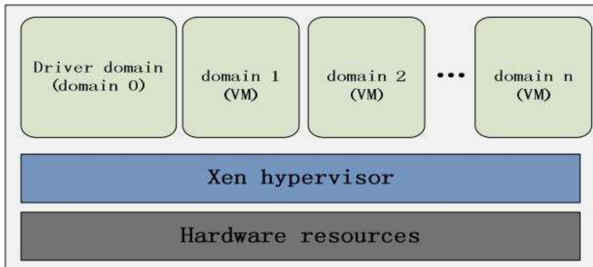
**Figure 2: The above figure shows the Xen Architecture.**
