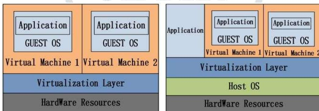
**Figure 1:** The above figure shows two types architectures of VMM.
