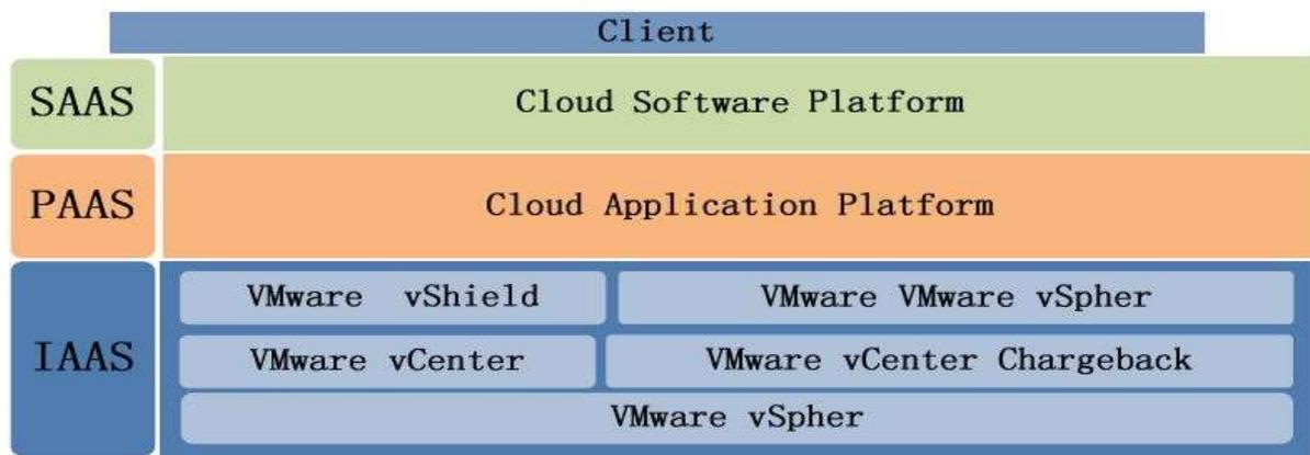
**Figure 3: The above figure shows the three-tier cloud-computing platform based on the VMware vCloud tools.**
