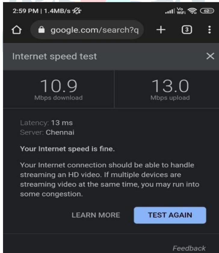
Fig.24 Results of Wi-Fi Router with Existing Antennas
