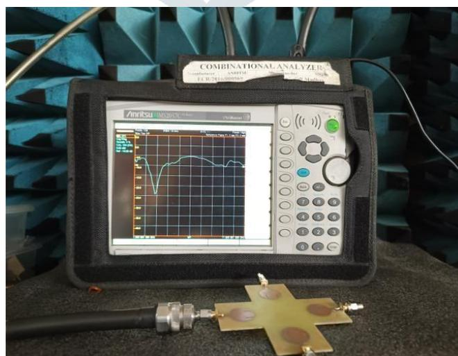
Fig.13 S11 Plot of Fabricated Antenna From VNA
