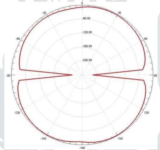
Fig.18 X plane radiation pattern at 10GHz
