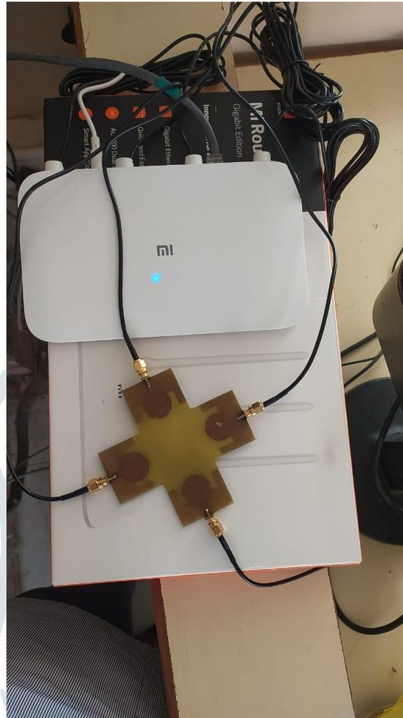
Fig.25 Wi-Fi Router with Proposed Antenna
