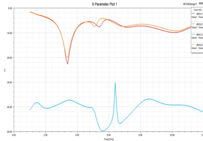
Fig.10 S parameters of 4Element Orthogonal MIMO Antenna.
