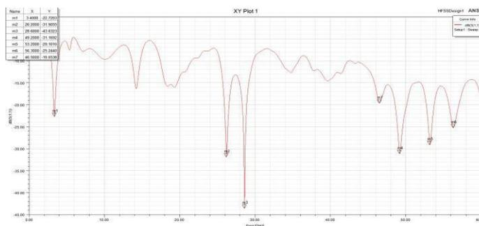
Fig.4 S11 Plot of Proposed 4 Elements Orthogonal Antenna.
