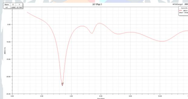
Fig.2 S11 plot of single pole antenna.
