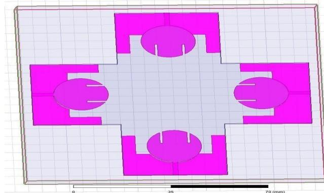
Fig.3 Proposed 4 Element Orthogonal Antenna.
