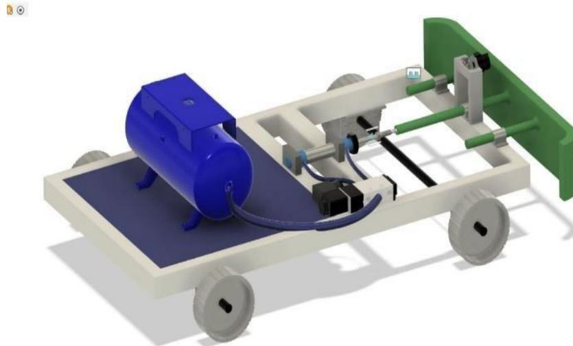
Fig.9 3D Model of Pneumatic Bumper System
