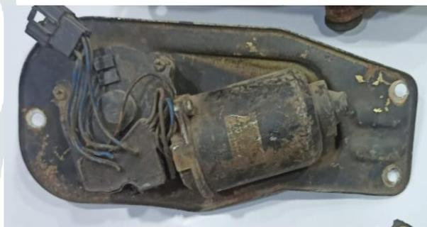
Fig.8 Wiper Motor
