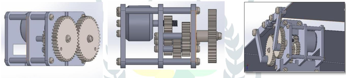
FIG. I GEARBOX ASSEMBLY
