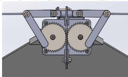
FIG. II DUAL GEAR CRANK MECHANISM
