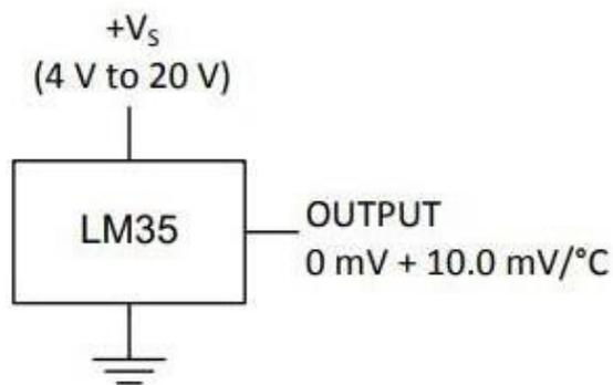
If the temperature is  $0^{\circ}\text{C}$ , the output voltage will also be  $0\text{V}$ . There will be an increase of  $0.01\text{V}$  ( $10\text{mV}$ ) for each degree of temperature increase. The voltage can be converted to temperature using the formulas below.
