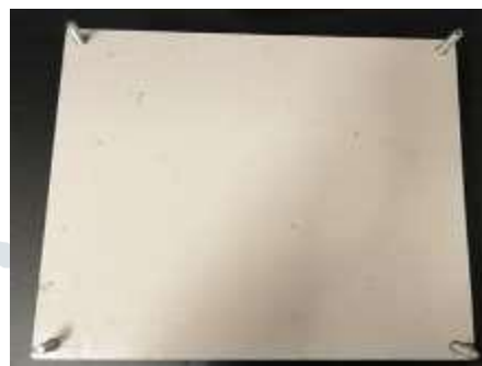
Figure 9. The piezoelectric tile that used for foot press activities
