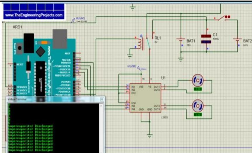
Fig.7. Serial Port Message For “SupercapacitorDischarged”
