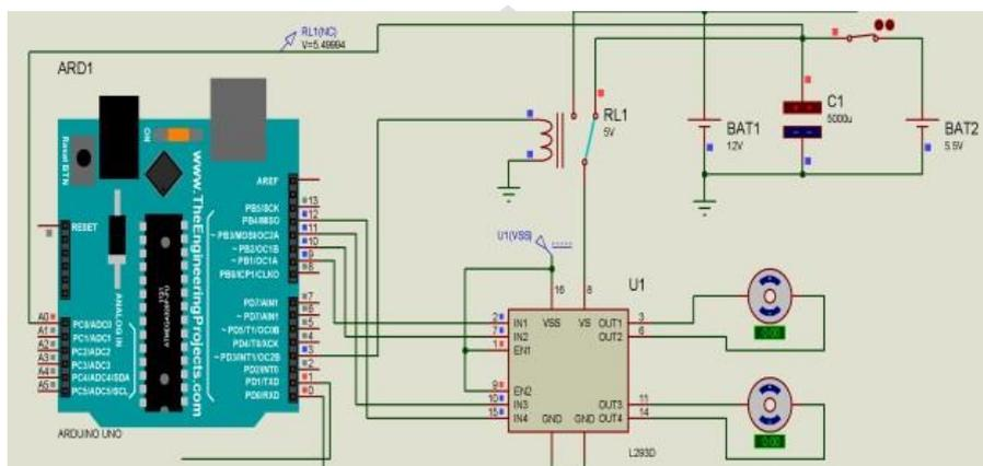
Fig.8. Capacitor Voltage Greater Than Reference, RelayOff
