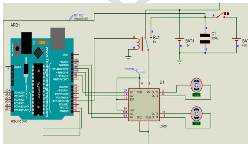
Fig.6. Capacitor Voltage Less Than Reference, Relay On
