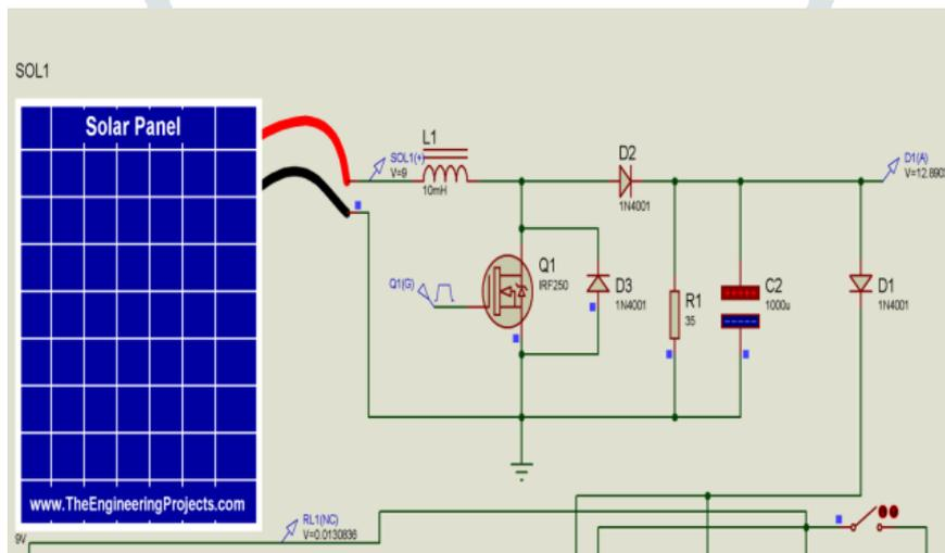
Fig.5.DC Output Voltage = 12.86  $\approx$  13V @ PV Voltage =9V
