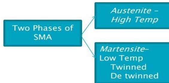
Fig. 1: Two Phases of SMA
