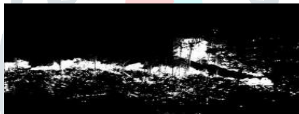
Fig. 7. The processed image on the Django web-app after applying the Sobel edge detection algorithm.
