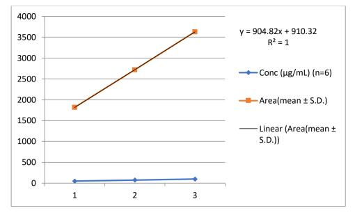
Fig.5: Graph of Calibration curve for Irbesartan
