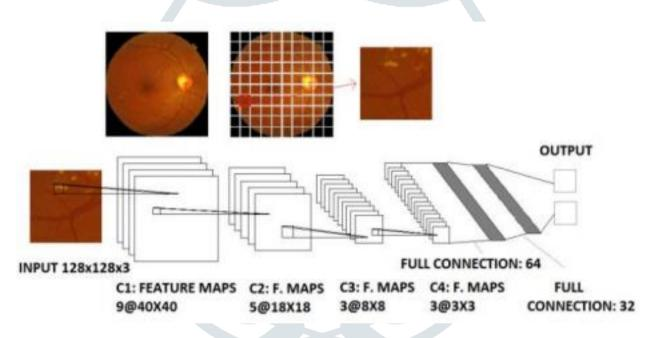
Fig 1 CNN architecture of the proposed method.
