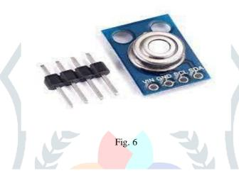
The MLX90614 is an infrared thermometer for non-contact temperature measurements. Both the IR sensitive thermopile detector chip and the signal conditioning ASIC are integrated in the same TO-39 can. Integrated into the MLX90614 are a low noise amplifier, 17-bit ADC and powerful DSP unit thus achieving high accuracy and resolution of the thermometer.
