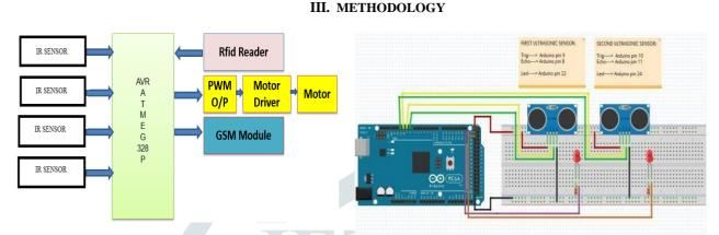
Car Parking System Using Arduino mega Designing, creating and delivering a main edge stopping innovation is called Smart stopping. It is a vehicle stopping framework that helps drivers locate an empty spot. Utilizing the IR sensors in each stopping space, it identifies the nearness or nonattendance of a vehicle. Brilliant Parking framework is demonstrated as a correct, strong and cost-effective approach to guarantee that street clients know precisely where empty car parking spots are.
