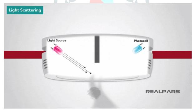
The light scattering smoke detector operates on the Tyndall effect; a photocell and light source are separated from each other by a darkened chamber such that the light source does not fall on the photocell.
