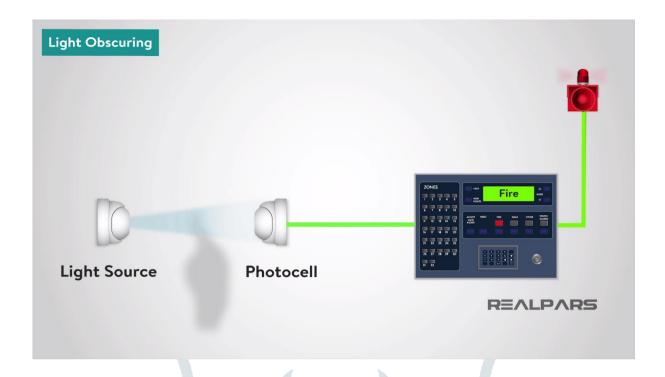
In the Light obscuring smoke detector, smoke interferes with a light beam between a light source and photocell. The photocell measures the amount of light it receives. The variation in photocell output, is being used to initiate an alarm.
