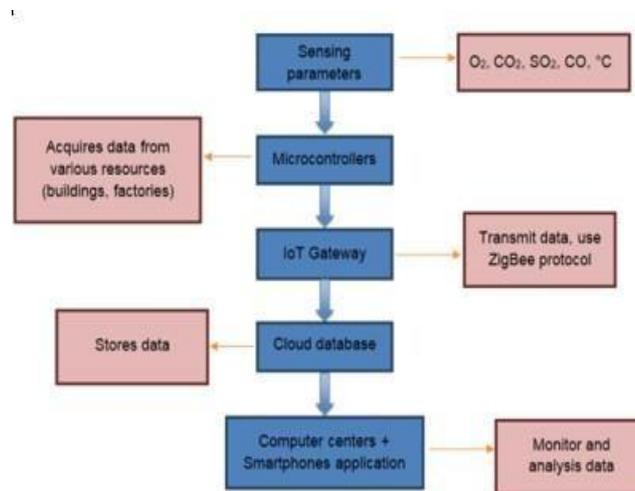
Fig. 2 Conceptual Block Diagram
