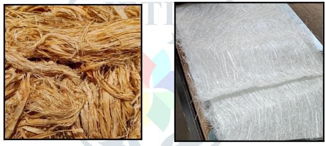
Fig. 2 Hemp Fiber NaOH Treated
