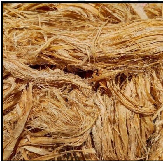
Fig. 2 Hemp Fiber NaOH Treated
