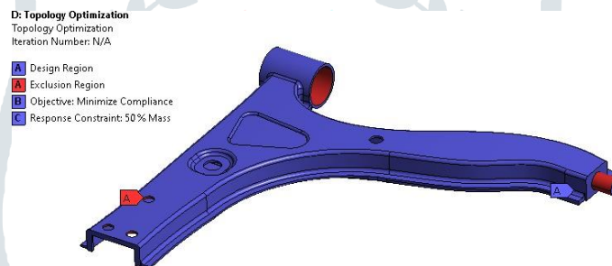
Fig 5. Boundary condition for topology optimization region
