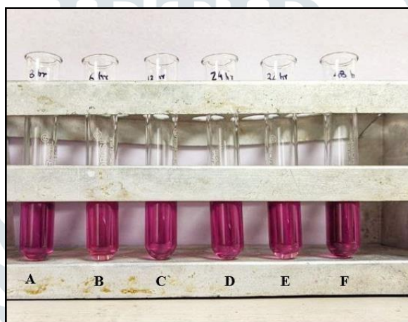
Fig 1.7 Representation of Spectrophotometric assay for Supernatant extracted from shake flask studies. 3hrs (A), 6hrs (B),12hrs (C), 24hrs (D), 36hrs (E), 48 hrs (F).
