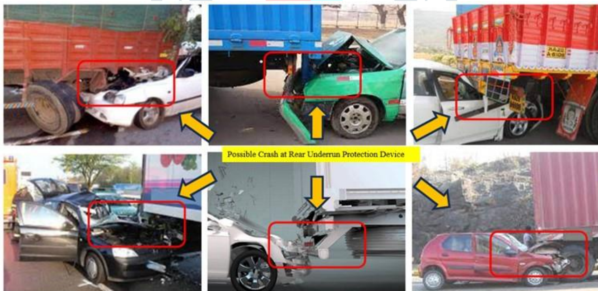
Figure 2. Possible Crash at Rear Underrun Protection Device (RUPD)
