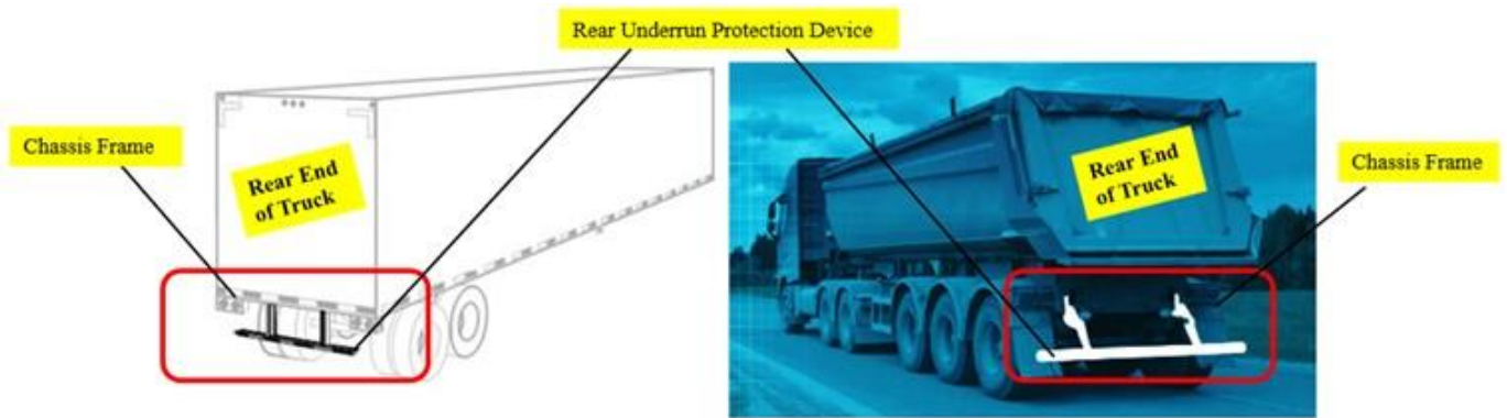
Figure 1. Schematic of Rear Underrun Protection Device (RUPD)
