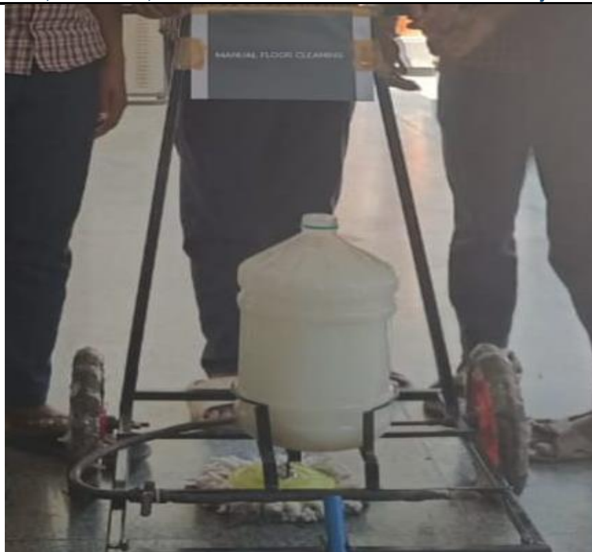
Fig 5. Automatic floor cleaner with a water tank fitted above
