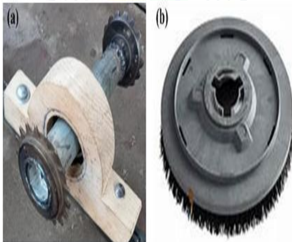
Fig 2. a) Roller bearings b) Pro-lite disc brush of 300mm diameter
