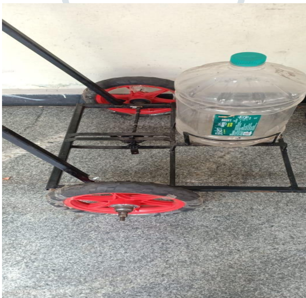
Fig 6 . 10 liters Water tank mounted on chassis
