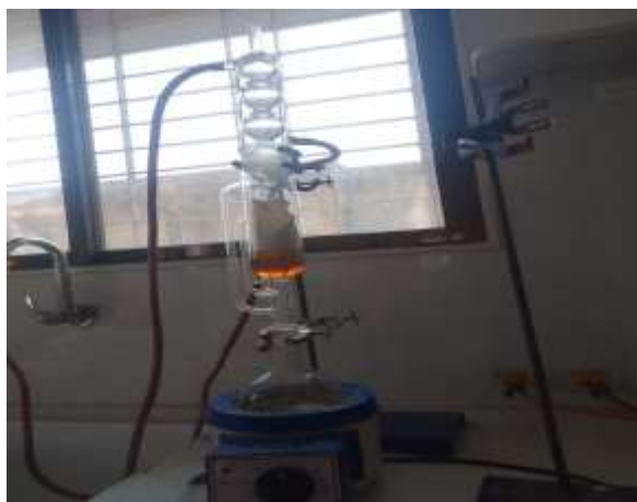
Fig. no. 1 Extraction of flavonoid by Soxhlet apparatus Fig No. 2 Phytochemical extraction
