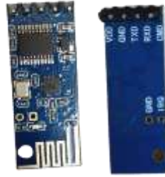
Fig 10: ZIGBEE MODULE(Transmitter & Receiver)
