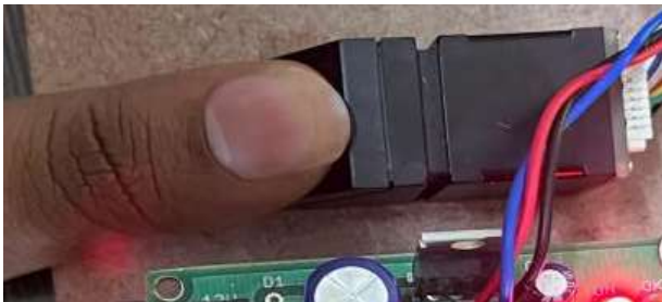
Step 2: Placing the finger on the fingerprint Scanner to verify discharge the line
