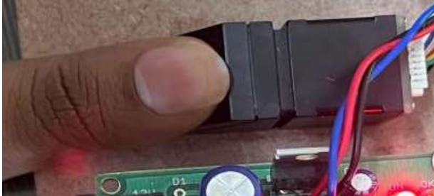
Step 2: Placing the finger on the fingerprint Scanner to verify to charge the line
