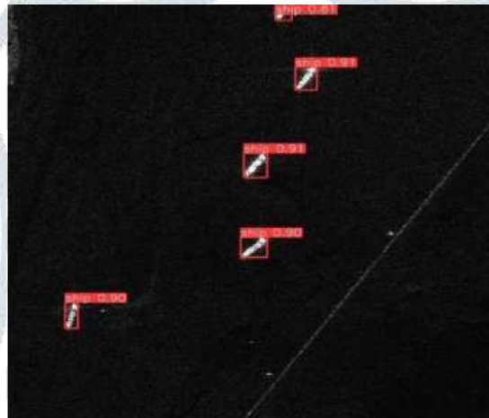
Figure 5: Ship Detection Results on SAR Image with Confidence Scores and Bounding Boxes
