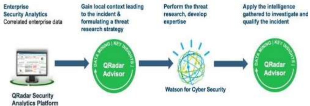
Figure 9: Stages involved in the working of IBM’s QRadar advisor with WATSON
