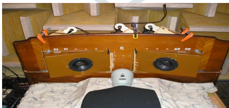
Fig. 2. Experimental setup of the snore ANC system
