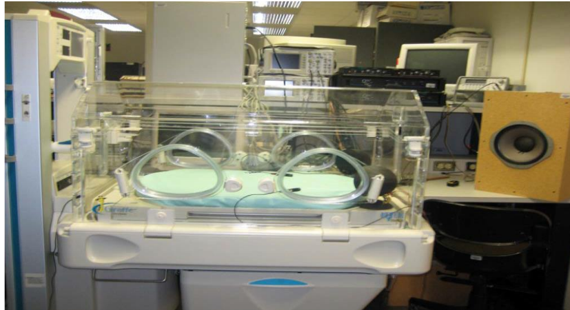
Fig. 6 ANC setup based on the GE Giraffe® incubator
