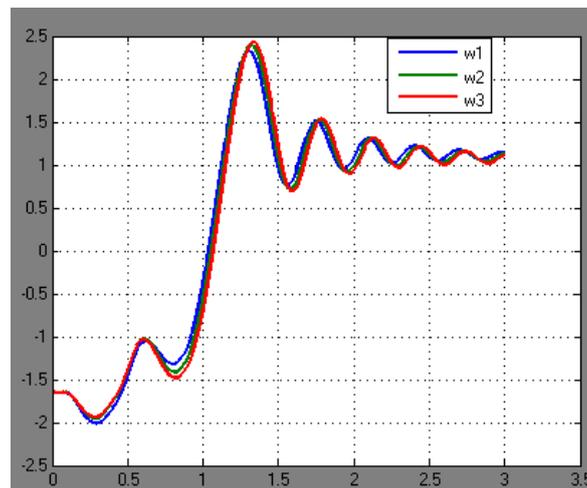
Fig. 9: Rotor angle deviation of G1 G2 G3 with feedback control system of VSCs with respect to time in secs
