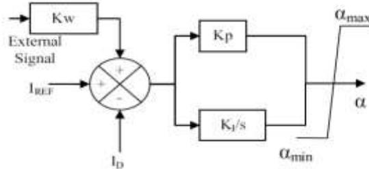
Fig. 7: Closed loop control of HVDC VSCs with Iref feedback
