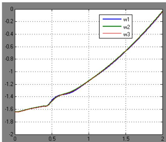
Fig. 3: Rotor angle deviation of G1 G2 and G3 with fault
