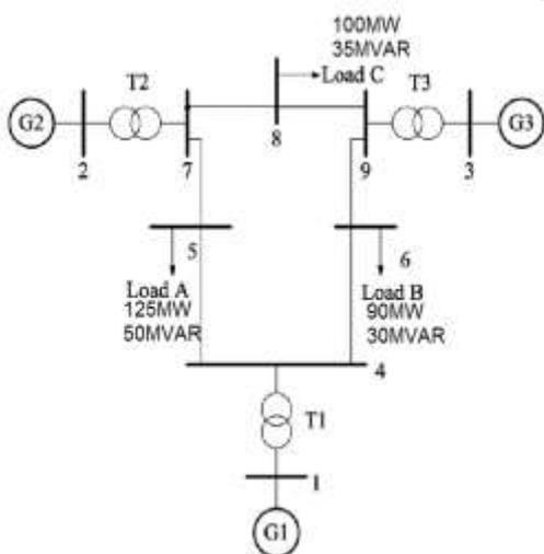
Fig. 1: IEEE 9 bus system single line diagram
