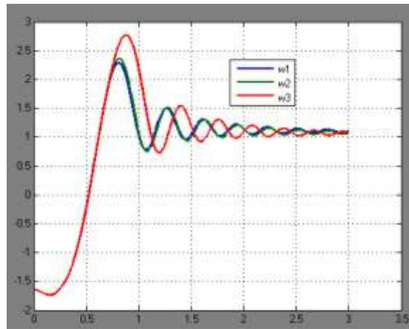
Fig. 6: Rotor angle deviation of G1,G2 and G3 with open loop HVDC transmission system
