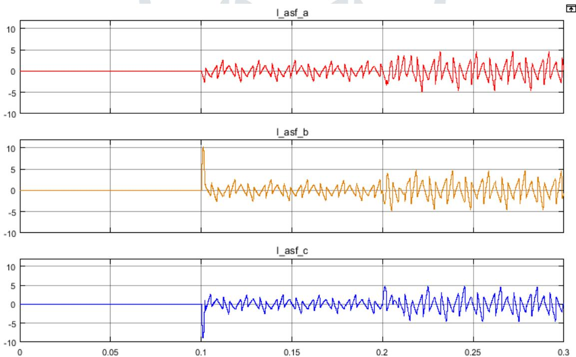
Fig. 9: Compensating Current supplied by ASF
