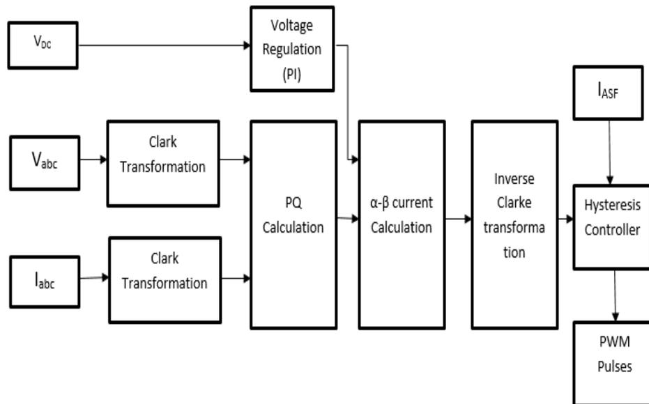
Fig. 2: Control strategy using Instantaneous real and reactive power(p-q) theory
