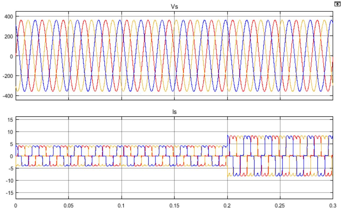
Fig. 8: Supply Side Voltage and Current waveform without ASF
