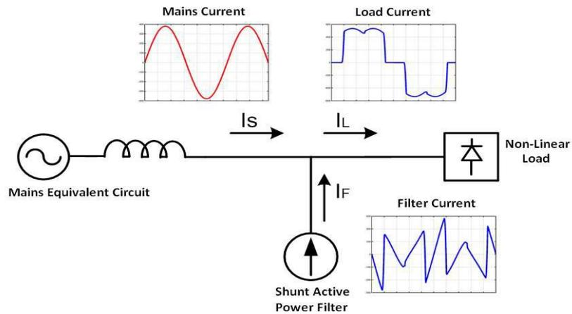
Fig. 1: Basic diagram of ASF
