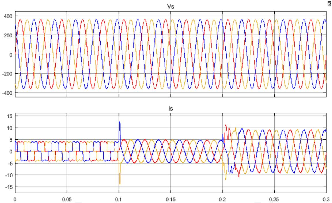
Fig. 10: Supply Side Voltage and Current waveform with ASF
