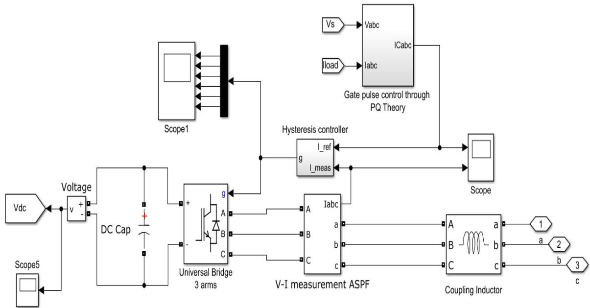
Fig. 6: subsystem of active shunt filter
