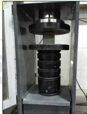
*Fig. 4: Compressive Testing Machine*
