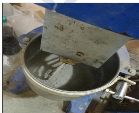
Fig. 1: Mortar Mixture Machine
