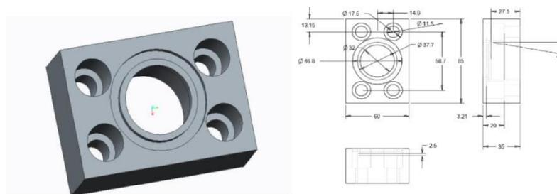
Figure 1 Flange and its Dimensions
