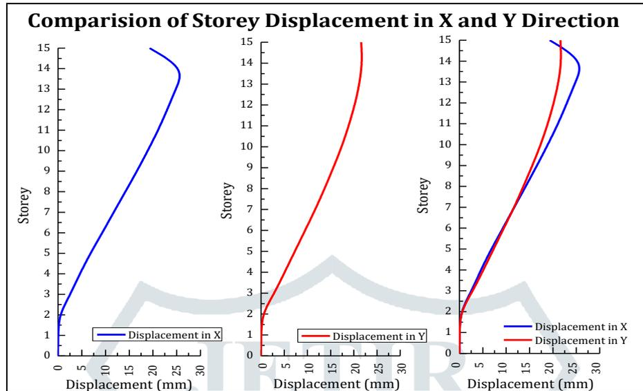
Fig. 4 Comparison of Storey Displacement
