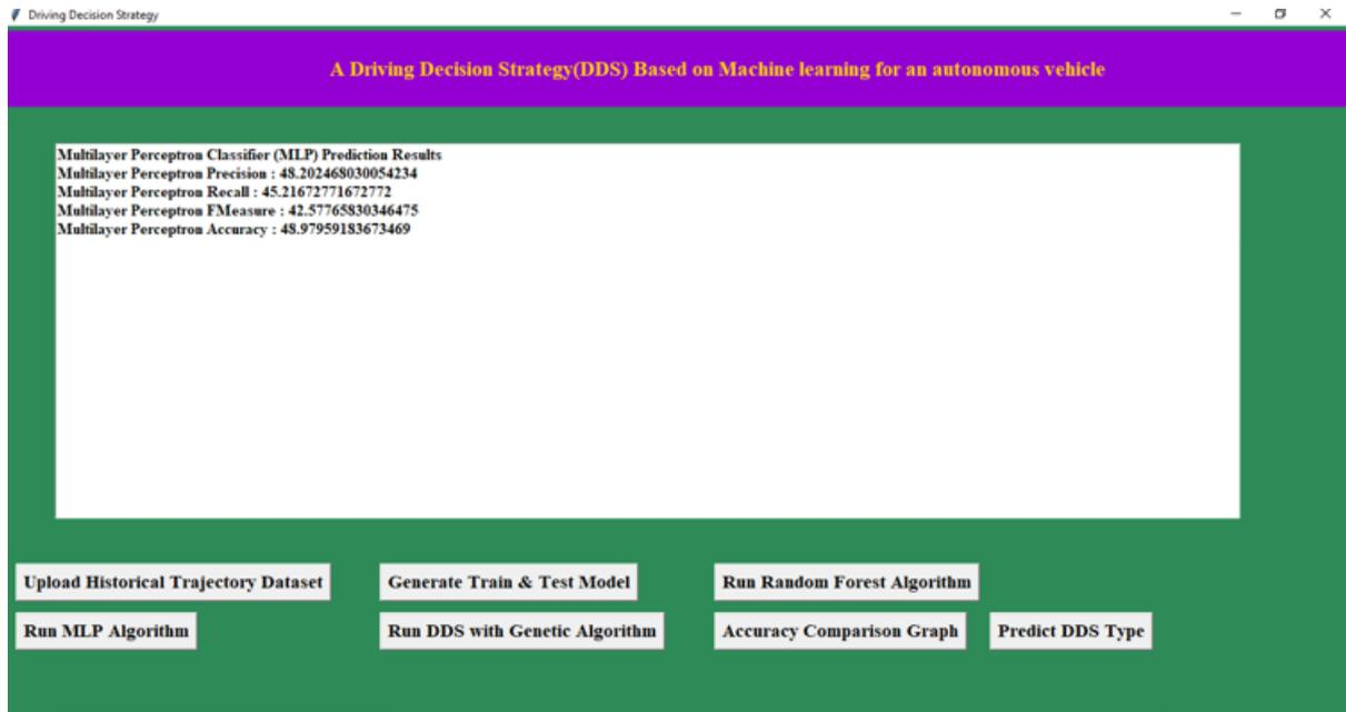
In above screen MLP got 48% prediction accuracy and in below screen we can see genetic algorithm code used for building propose DDS algorithm
