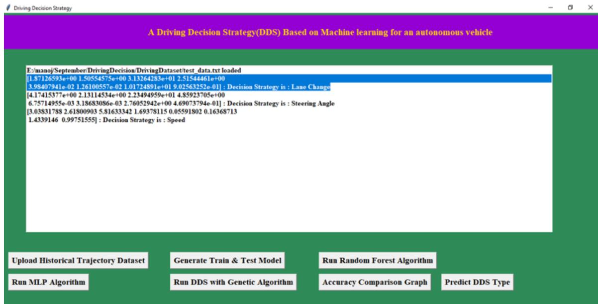
In above screen in selected first record we can see decision is Lane Change and for second record values we got decision as 'steering angle' and for third test record we got predicted value as vehicle is in speed mode.
