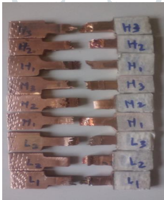
Figure 3.10 The tensile specimens after the test in (before the taste shown in appendix I)
